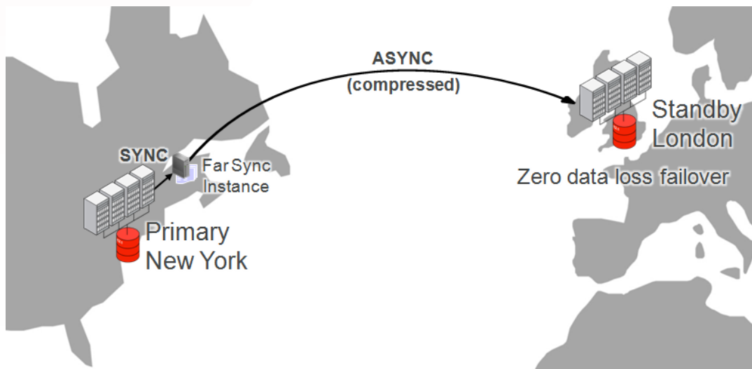
Figure 8: Active Data Guard Far Sync – Zero Data Loss Protection at any Distance
